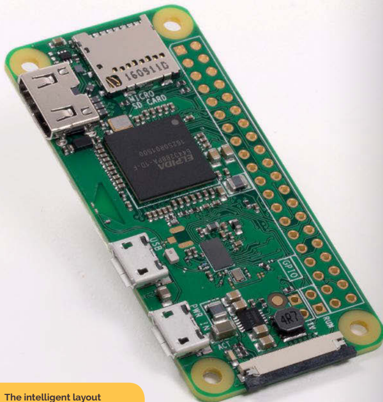
The intelligent layout enables all the circuitry to be placed on one side of the PCB, keeping the cost down
